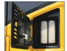
External air conditioner filter
