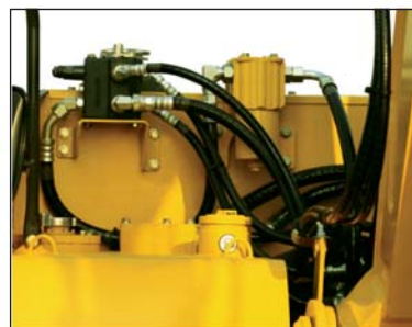
Selector valve & additional filter Selector valve for breaker and crusher
